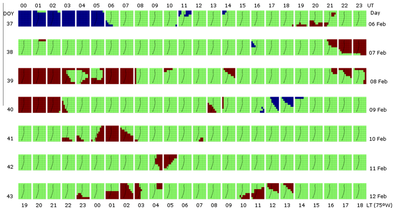
Fig. 6. Times for which TEC (regional representation) at 72 grid points, over an area covering the whole ~400 km earthquake rupture zone (37.0–30.0°S; 67.0–75.0°W), are smaller than the reference lower boundary (previous 15-day running median minus interquartile range – blue) and larger than the reference upper boundary (previous 15-day running median plus interquartile range – red) from 6 to 12 February 2010 (DOY 37–43). (thin black line) Approximate coast line. (For interpretation of the references to color in this figure legend, the reader is referred to the web version of this article.)
